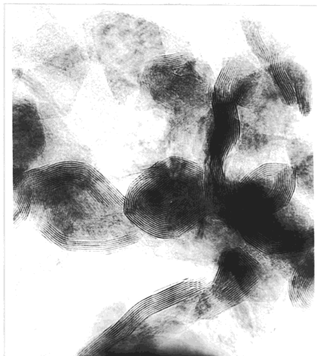
Figure 1. TEM image of the as-prepared powder. Scale: 1 cm = 9 nm.
